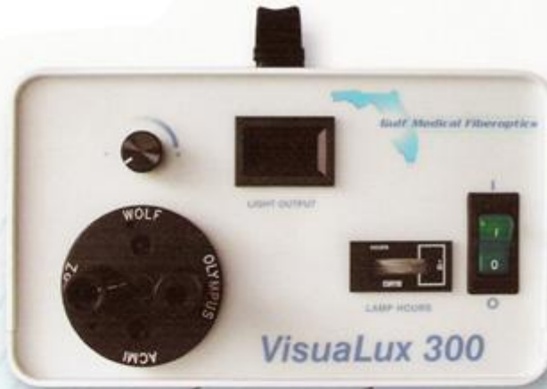
Multi port turret, front panel includes light output LED and re-settable lamp timer.
